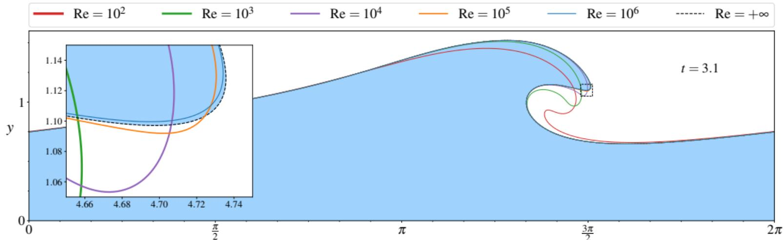
$Re = +\infty$  simulations (i.e. Euler solution) computed with the numerical methods of
